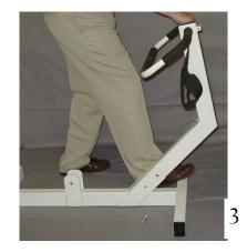
STEP 2: **HANDLEBARS** Hold the handlebar horizontal and place the bolt through the top bracket hole. STEP 3: Once you have the bolt through both the bracket and the handlebar, flip the handlebar up and put the other bolt through. STEP 4: When you tighten this bolt, stand in front of the machine, leaning against the handlebar so that you have pressure toward the back of the machine. (as shown) Tighten the bottom bolt first, STEP 5: followed by the top bolt.
