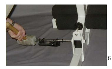
STEP 8: **SEAT POST** When you place the long axle through the upright, if you are right handed, put it in on the left side of the machine, standing behind the machine. DO NOT USE A HAMMER! USE A RUBBER MALLET. Slide or shove the axle through. Place another 0-ring, pedal, o-ring and finally the collar.
