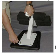
STEP 1: **SEAT** Place seat, cushion side down, on floor. Now place seat bracket on top of seat and insert and tighten the four seat screws, with washers, with the allen wrench provided. Attach the seat with the small end of the seat toward the front upright, with the wide end toward the back of the machine. (as shown)
